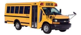
**Type B:** A Type "B" school bus is constructed utilizing a stripped chassis. The entrance door is behind the front wheels. This definition includes two classifications:
