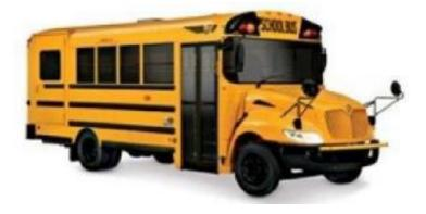
**Type C**: A Type "C" school bus is constructed utilizing a chassis with a hood and front fender assembly. The entrance door is behind the front wheels. This is also known as a conventional school bus. This type also includes cutaway truck chassis or truck chassis with cab with or without left side door and a GVWR greater than 21,500 pounds.
