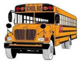
**Type D**: A Type "D" school bus is constructed utilizing a stripped chassis. The entrance door is ahead of the front wheels. These are also known as rear engine transit style school buses.
