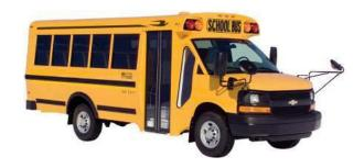
**Type B:** A Type "B" school bus is constructed utilizing a stripped chassis. The entrance door is behind the front wheels. This definition includes two classifications:
