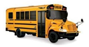
**Type C:** A Type "C" school bus is constructed utilizing a chassis with a hood and front fender assembly. The entrance door is behind the front wheels. This is also known as a *conventional school bus*. This type also includes cutaway truck chassis or truck chassis with cab with or without left side door and a GVWR greater than 21,500 pounds.
